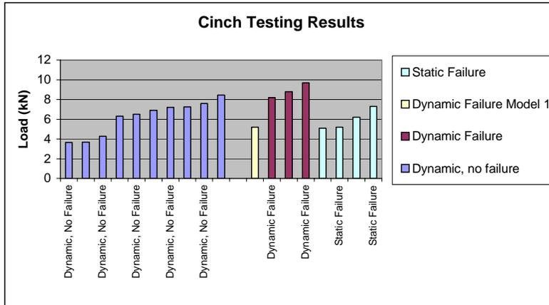
**Figure 14: Static versus dynamic failure for Cinch.**
