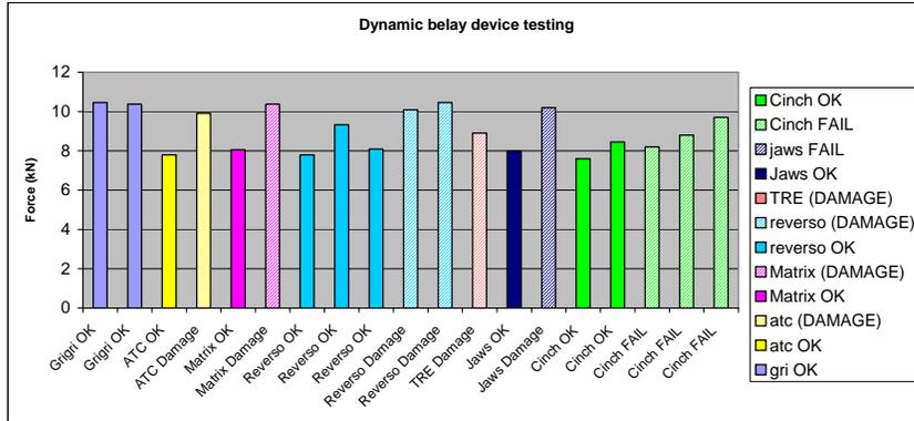
**Figure 12: Dynamic Results for different belay devices.**
