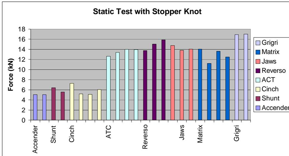
Figure 11: Static failure force for belay devices.
