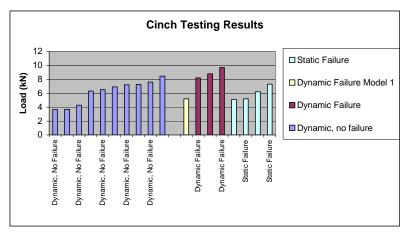
Figure 14: Static verse dynamic failure for Cinch.
