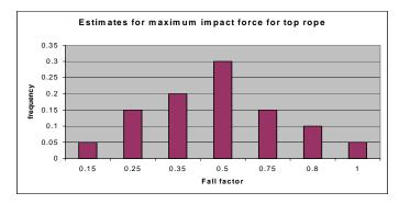
*Figure 8: Assumed* fall factor distribution when falls are limited to a fall factor less than 1.0.
