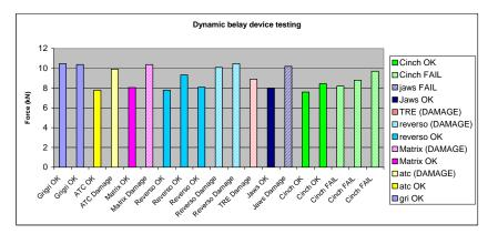
Figure 12: Dynamic Results for different belay devices.
